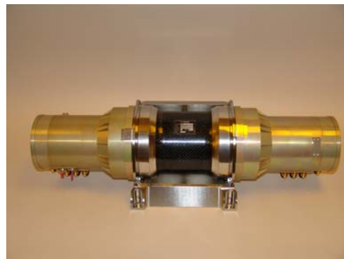
FIGURE 3. A BGO detector in its Ti holding structure.
